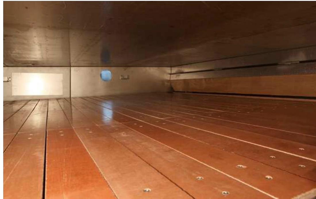
Refractory material for direct loading of product onto belt
